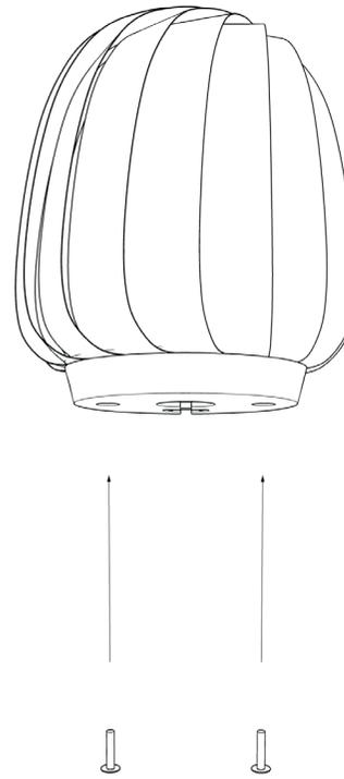
3) Insert the screws into the base to secure the lampshade
