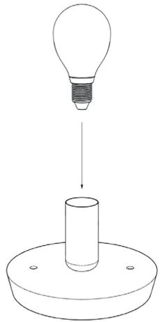
1) Insert a lightbulb in the E14 socket on the base
